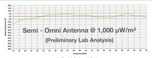
±5dB, 20GHz-40GHz 3dB Response Time: < 50 μs
