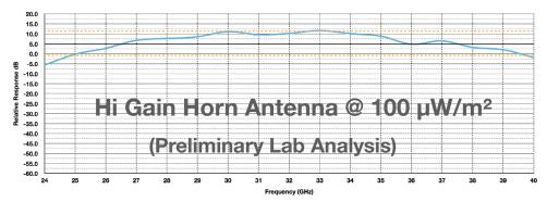
±6dB, 25 GHz - 40 GHz 3dB Response Time: < 50 μs
