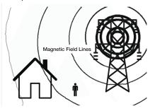
AC Magnetic Fields: concentric rings radiating from a source, which decrease with distance. Measurement units are expressed in milliGauss (mG) or in nanoTesla (nT).
