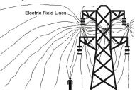
AC Electric Fields: jagged field lines lines from a radiant source, which travel to places of lower electrical potential or to ground. Measurement units are expressed in Volts per metre V/m.
