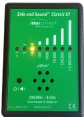
The Safe and Sound Classic III is 3rd party tested and 5G ready. It is ideal for those with no technical experience. Unlike any other meter in its price range, it utilizes the same measurement technology as the Safe and Sound Pro II for a fraction of the cost. It is a simple to use detector for radio frequency / microwave radiation, with exposure levels indicated by colored LEDs. This device offers readings from 200MHz to 8 GHz, which are sensitive below 1  $\mu\text{W}/\text{m}^2$ .
