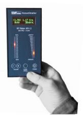
Ideally hold the meter as shown in the picture. Try to keep the Acoustimeter at least 30cm away from your body when taking readings. Keep your hands towards the bottom of the instrument.
