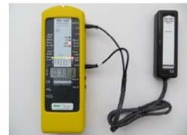
In order to put the sensor into operation, switch on the NFA, connect the sensor (or vice versa) and shortly press the button "Rec.". The display will show the magnetic flux density in the preset unit (G or  $\mu\text{T}$ , mind the LED "x1000" if applicable). The LEDs on the sensor will be lit.
