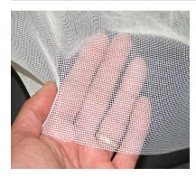
Swiss Shield New Daylite is a decorative, highly transparent, open mesh polyester shielding fabric with excellent air and light penetration
